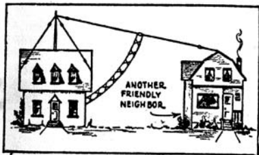
Fig. 23. Shows short-wave antenna with transposed lead-in erected over vacant lot, if your neighbor will permit you to anchor the antenna to the roof of his house.
