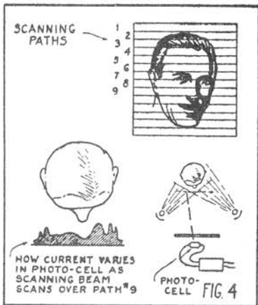
How image is scanned and how light varies along each scanning path
