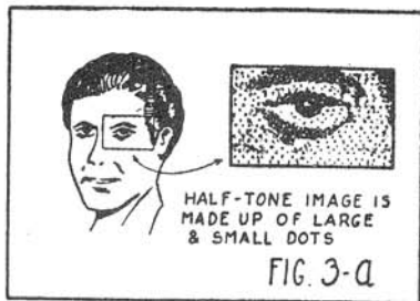
Half-tone images are made up of a series of dots
